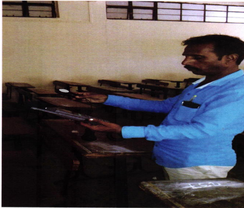
Illumination Monitoring in Classroom
