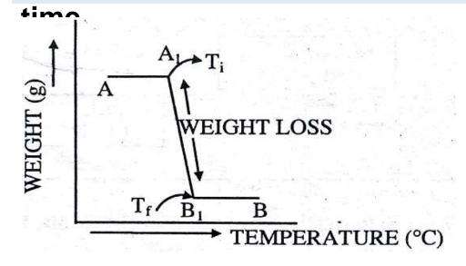
1.Horizontal portion of the plot indicate the temperature range in which there is no weight loss (Portion A to A1)
