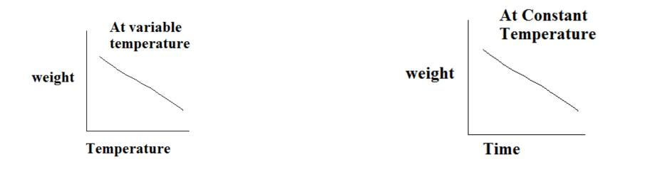
At variable temperature weight is plotted against temperature
