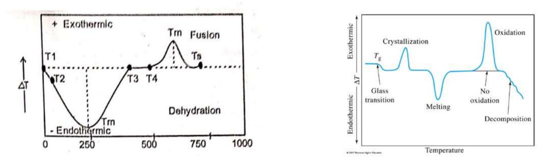
Exothermic peaks gives idea about crystallization and fusion process. Endothermic peaks gives idea about dehydration, melting etc.
