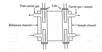
Two filaments are connected to two arms of Wheatstone bridge.
