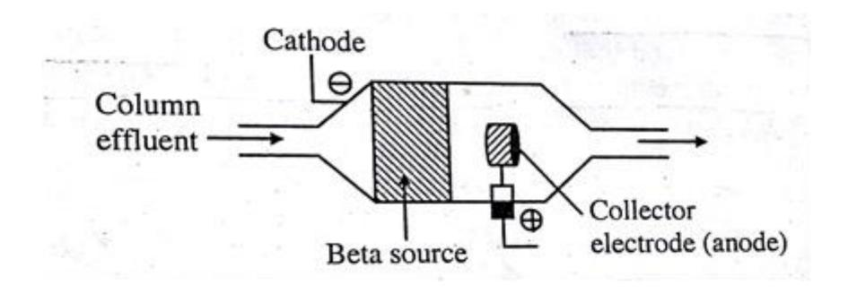
**Construction:** Detector consists of metal box acting as cathode (negative electrode). Inside this box there is beta ( $\beta$ ) emitting source (i.e., <sup>3</sup>H or <sup>63</sup>Ni). Collector electrode act as anode (Positive electrode).
