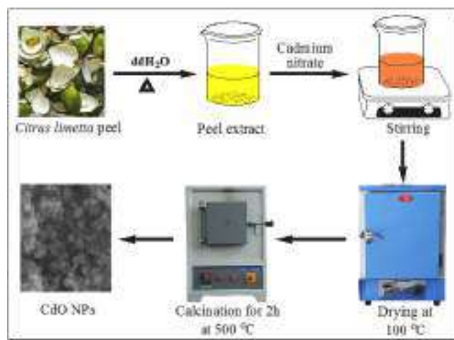
Fig. 2. A pictorial depiction for the bio-inspired fabrication of CdO NPs from Citrus limetta peels extract.
